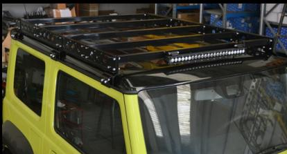
All plates are 5mm thickness, squared brackets in 35x35x3, 6 fitting points to the roof, easy fit on top; made up in steel, black powder coated
