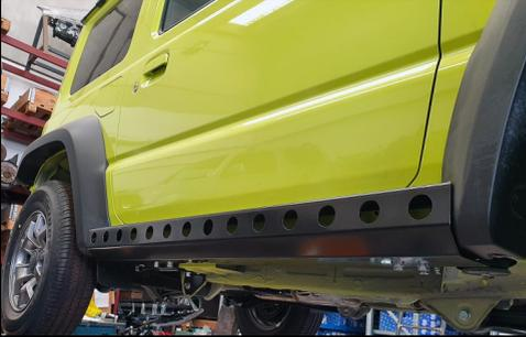
Thickness 6mm, folded and reinforced inside, very heavy duty and great looks for Jimny; black powder coated
