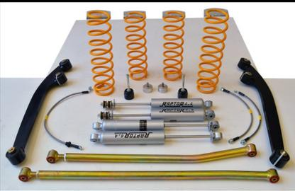
"Complete Trial" is the most complete Raptor 4x4 suspension system for Suzuki Jimny, which increase a lot the twist, and get good driving on road and fast offroad to.
