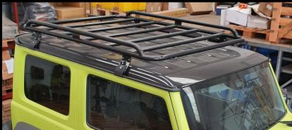
Tube 35x2 with 4 fitting points to the roof; black powder coated
